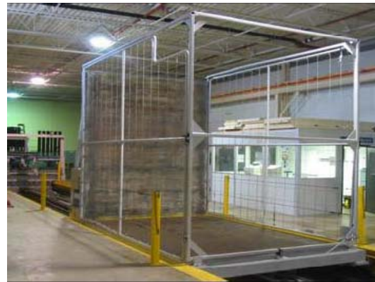
Real World Rail Impact Tester Full scale simulation of rail car coupling ("humping")
